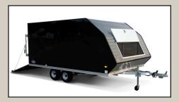
The AmeraLite Blast...comes with a rear ramp door and front access door standard. Every unit is framed for an optional side door. Ramp doors have double automotive bulb seals -locks out dust, moisture, and road grime for superior protection over single weather strip used by other manufacturers.
